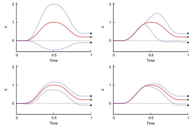
Fig. 2. Comparison of goal adaption between original (top row) and new (bottom) form of dynamic movement primitives. Graphs show a sample movement  $x(t)$  to the original goal (red solid curve) and its adaptation to new goals (blue dashed curves). As the time of goal switch, we chose either 0 (left column) or 0.4 (right column).
