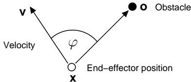
Fig. 4. Definition of the steering angle  $\varphi$ .
