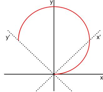
Fig. 1. Original form of dynamic movement primitives depends on choice of coordinate system. Two coordinate systems are plotted  $(x, y)$  and  $(x', y')$ . In the primed coordinate system, start and end point of a sample movement (red curve) are on the  $y'$ -axis. In this case, the motion generation will fail to produce the desired trajectory, since the motion will be restricted to  $x' = 0$ .
