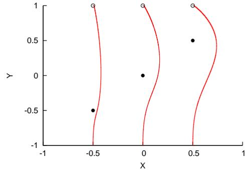
Fig. 6. Obstacle avoidance in 2D space. Three separate movements are shown, each with a different obstacle position (black dot). Goal positions are marked by circles. Here, for simplicity,  $\mathbf{f}(s) = (\mathbf{g} - \mathbf{x}_0)s$ ; thus, terms depending on  $s$  vanish. The goal positions were shifted by 0.01 to the right from the lines going through start and obstacle positions.
